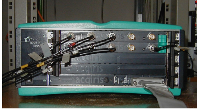
Figure 4.7: Crate with two Acqiris digitiser modules.
