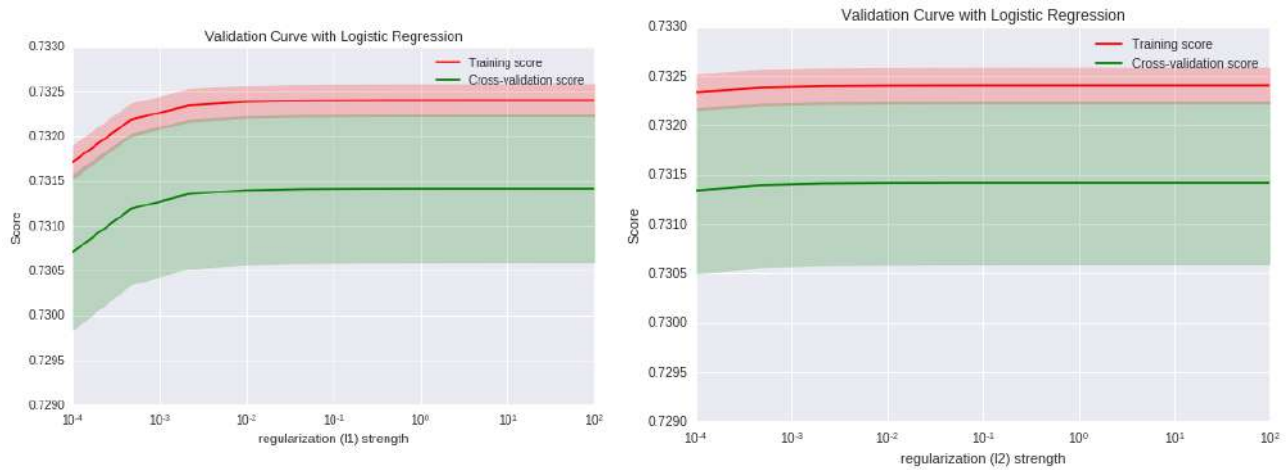
Figure 4.8.2: Logistic Regression validation curves. The plots present the impact of L_1 (left) and L_2 (right) regularization on classifier performance.
