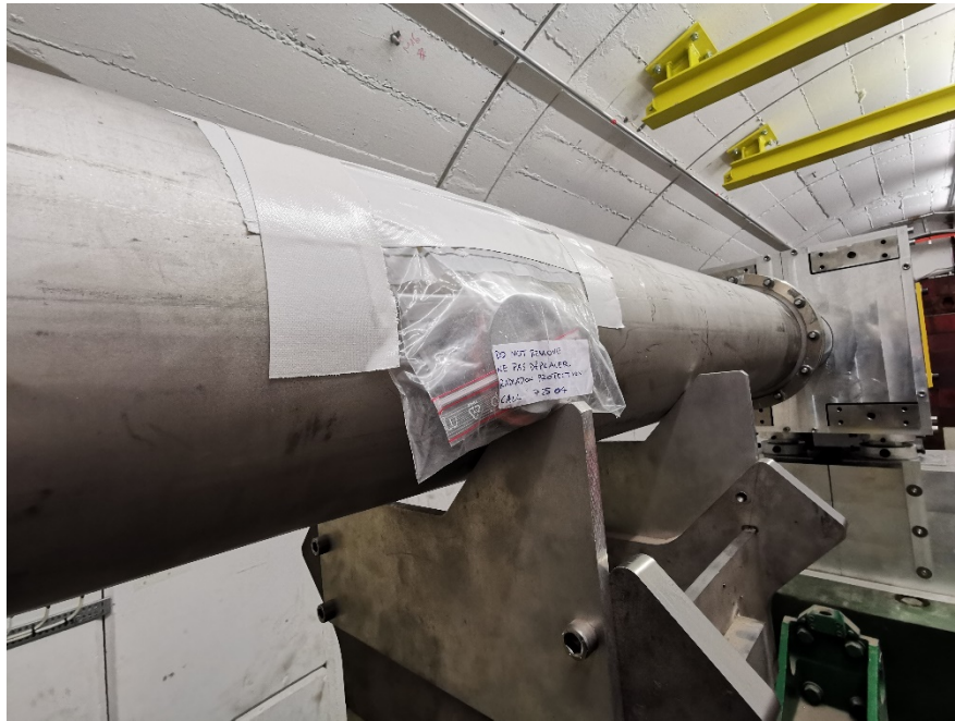
Figure 5.7: Positioning of the sample upstream the permanent magnet.
