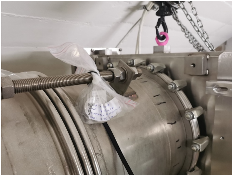
Figure 5.3: Positioning of the sample upstream the 1st collimator.
