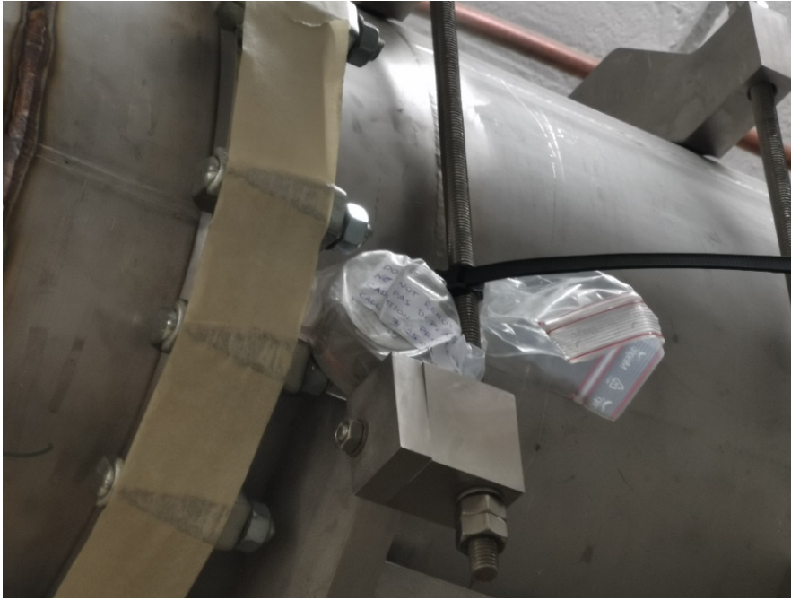
Figure 5.5: Positioning of the sample upstream the 2nd collimator.
