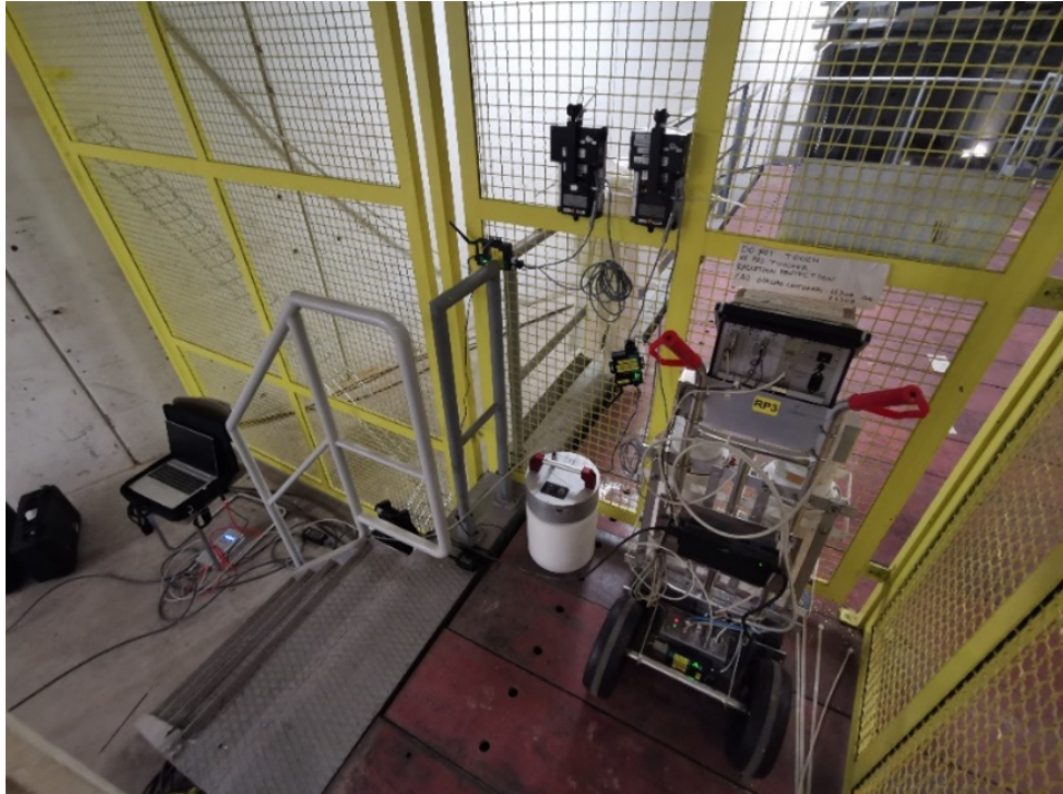
Figure 4.1: Portable detectors installed ISR8: the LUPIN (white cylinder) and the IG5 trolley (on the right hand side with respect to the LUPIN) with the hydrogen- and argon-filled high-pressure ionization chambers.
