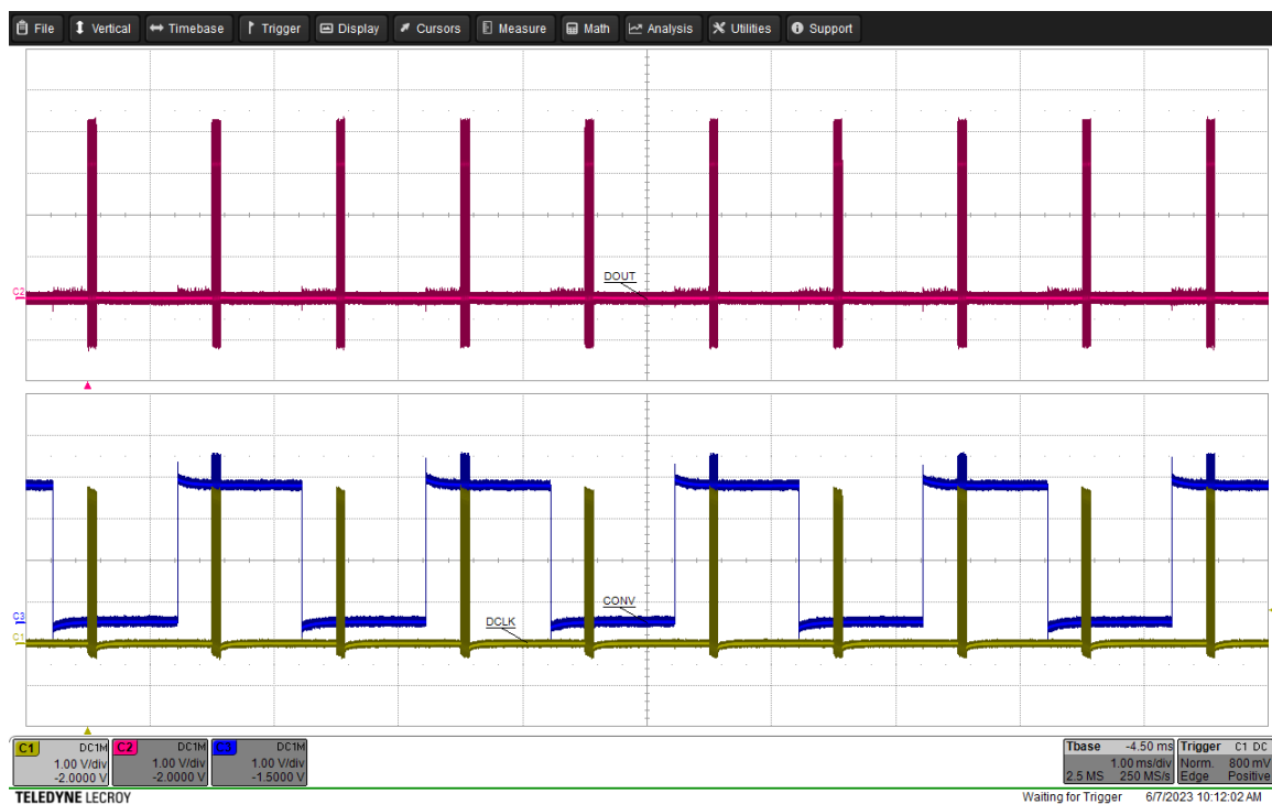
FIGURE 4.7: DDC232 timing diagram with reference of CONV signal
