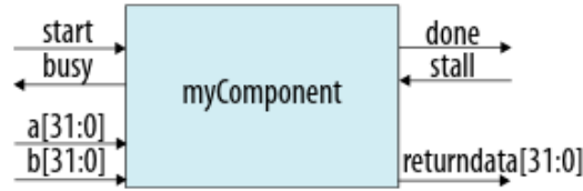
Figure 3.22.: Schematic of the data interfaces of an HLS streaming component.
