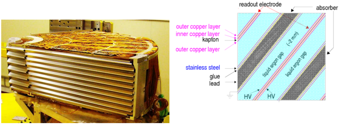
(a) Photo of an electromagnetic end-cap module, (b) Schematic of a cell of electromagnetic calorimeter [1]
