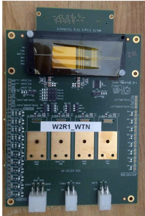
Figure A.8: Picture of a MALTA chip. The pixel matrix is the 2 \times 2 \text{ cm}^2 squared sensor at the top of the board, protected with the yellow tape. August 2020, photo credits: MGF.
