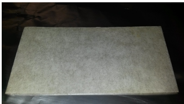
Figure 18: 100 mm × 50 mm and 1 mm thick PEEK sample sheet.
