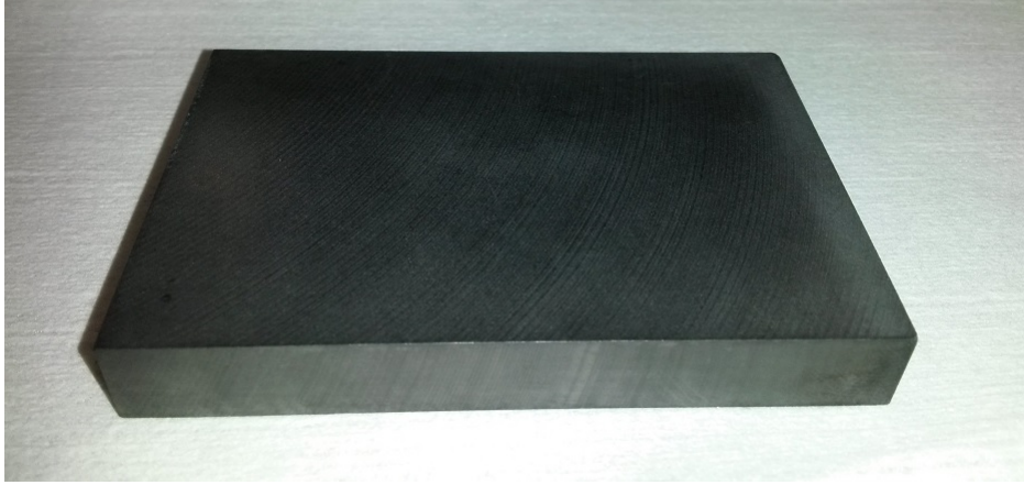
Figure 23: One of the four identical graphite samples. Sample dimensions: 75 mm \times 50 mm, thickness 10 mm.
