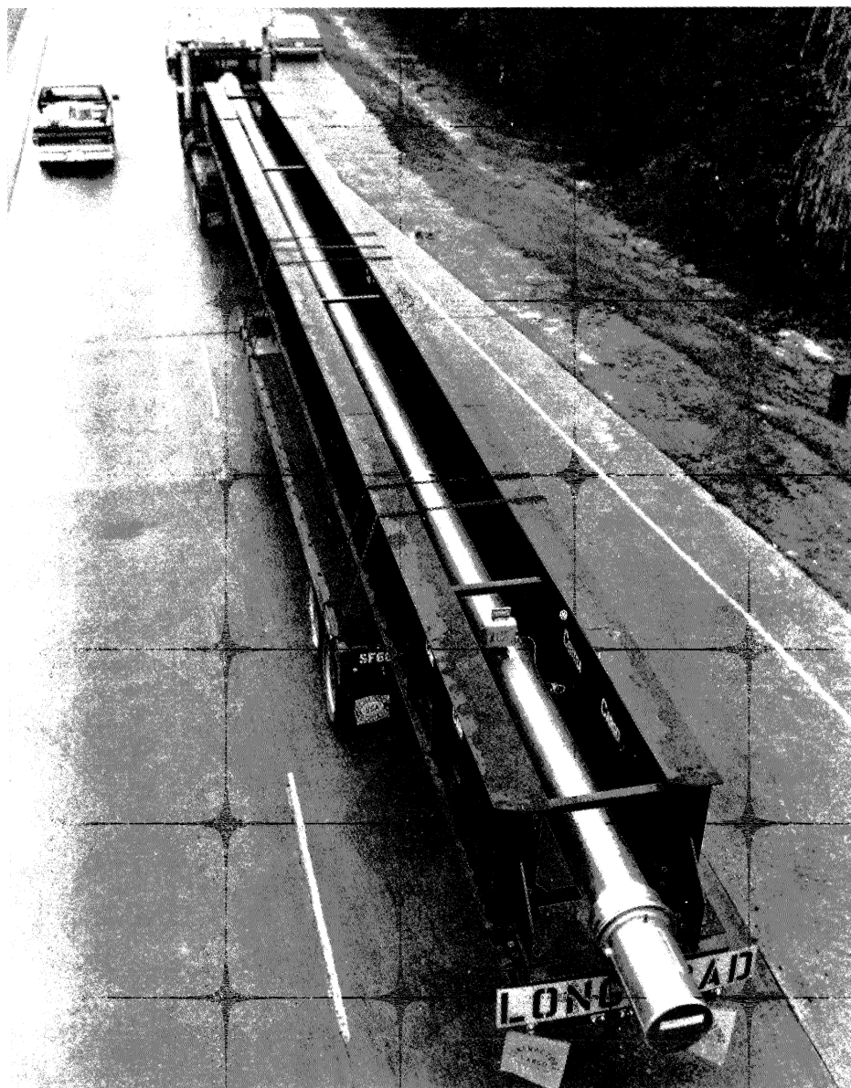
'Supertex' on its way to the Texas Accelerator Center. 28 metres long, it is the longest superconducting magnet to be made. The small instrument visible on the top of the magnet records road shocks.
