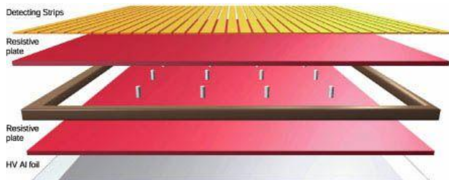
Figure 1: Basic Construction of an RPC detector
