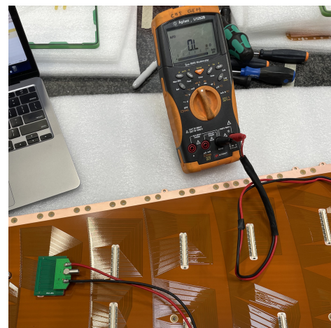
Figure 28: Short-circuit test setup, with the multimeter measuring resistance between strips and ground.
