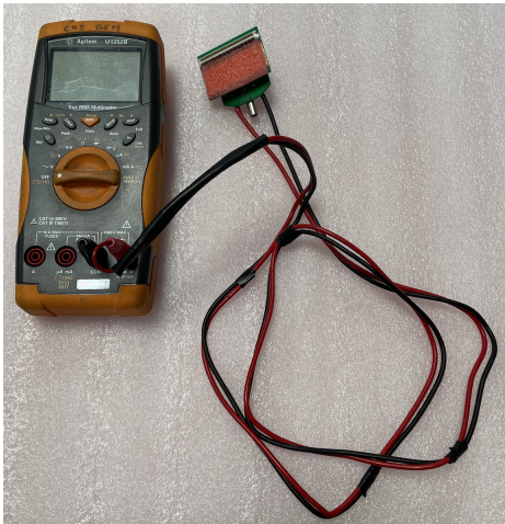
Figure 27: Multimeter and HRS connector used for short-circuit testing.
