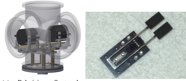
(a) Polarizing Sextupole, with spacing between the two halves. (b) CH-10 Tuning Fork Chopper.
