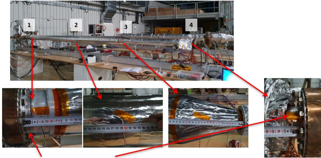
Figure 14: PT1000 Sensors on HF-CT2 before bakeout
