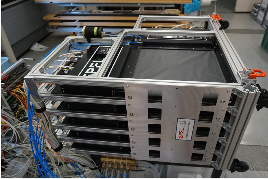
Figure 2.12: SND@LHC SciFi tracker with five stations [16].
