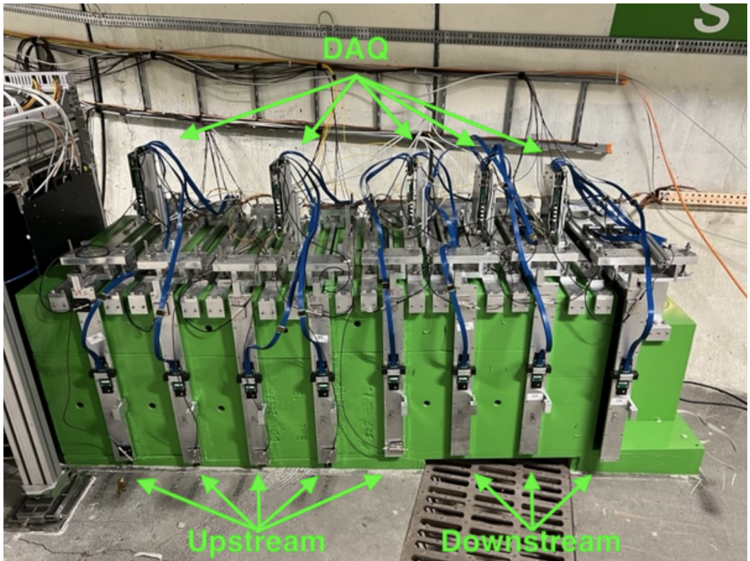
Figure 2.16: US and DS stations of the SND@LHC muon system [16].
