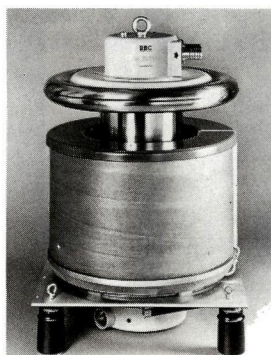
Special high-vacuum tetrodes for fast DC switching and control up to 170 kV, 120 A. Switching times in the order of \mu s. Integrated x-ray shield, SF 6 insulation and antiparasitic damping.
