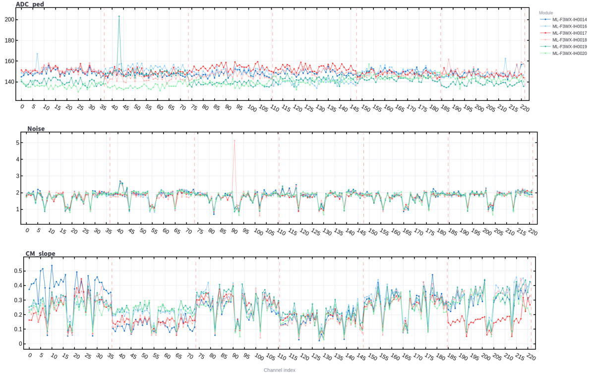
Figure 6.11: Monitoring plots showing the pedestal mean (top), noise (middle) and common mode slope (bottom) for the six modules from the first two layers in the 2024 beam test. Each point corresponds to an individual channel, with different colours representing different modules. These quantities are obtained from dedicated pedestal runs. The CM slope indicates the degree of correlation with common mode noise and is particularly relevant for precise signal extraction in MIP analysis.
