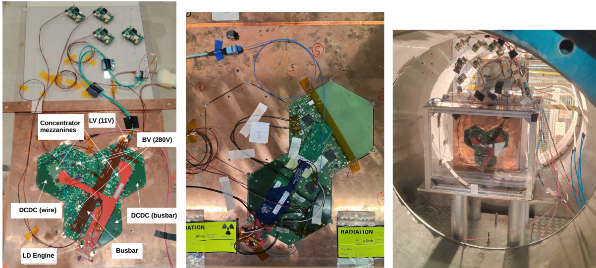
Figure 5.9: Photographs of different layers of the setup. Left: front/back train (3 low-density modules) with electronic components (concentrator mezzanine, low voltage power supply, DCDC bias voltage power supply and busbar). Middle: additional train featuring a high-density module with a partial bare hexaboard and partial concentrator mezzanine. Right: System inside the magnet with all the components from Figure 5.8 connected.
