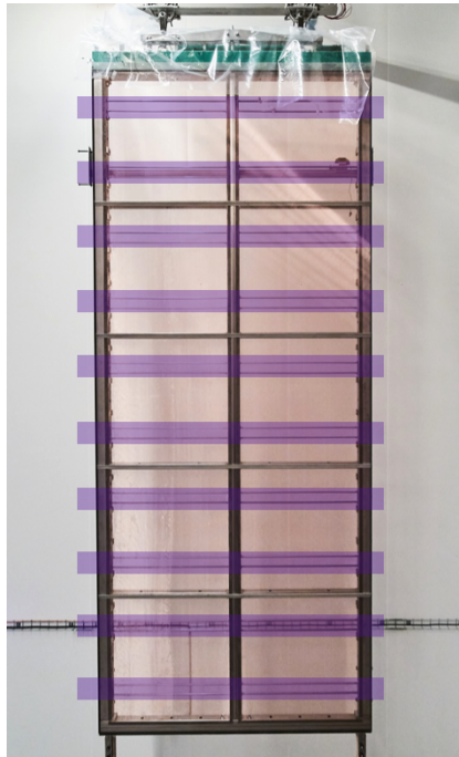
Fig. 5.8 Anode plane assembly (APA) example. The 10 photon detectors are highlighted with thick horizontal purple lines. Source: https://cds.cern.ch/record/2280729 .
