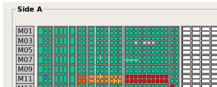
Figure 6: VELO Dashboard panel with LEDs indicating an error.
