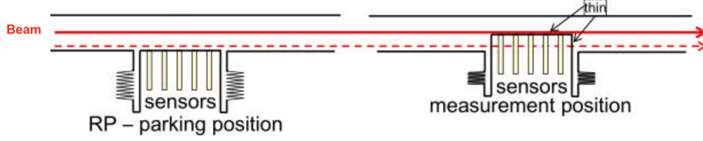
Figure 4.2: A vacuum chamber which houses the detectors is attached to the beam-pipe by means of bellows and the deformation on the bellows bring the detectors as close as possible to the beam line.
