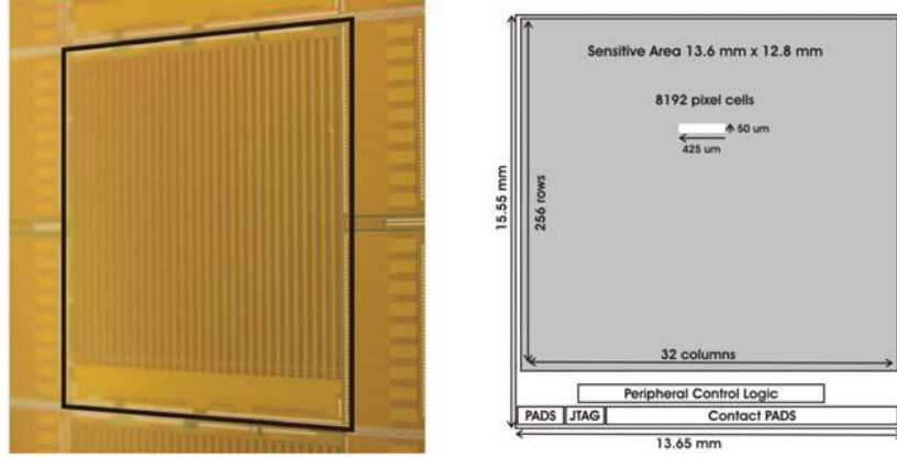
Figure 2.11: SPD readout chip ALICE1LHCb [25].
