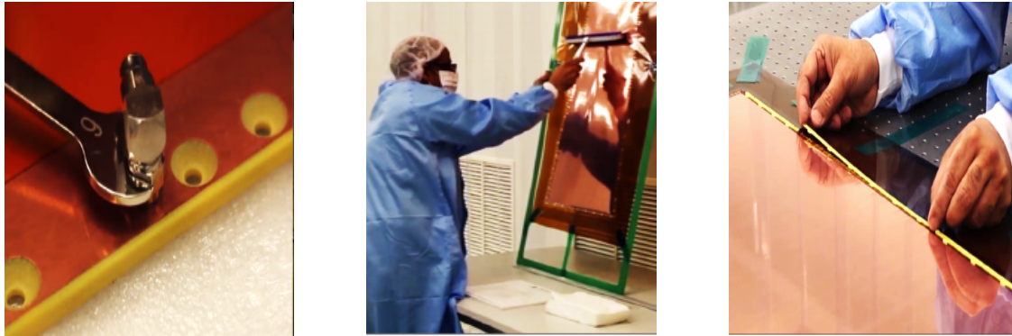
Figure 4. Left: Fixing the gas connector onto the readout board, Middle : Cleaning of the GEM foil with the anti-static roller, Right : Placing the internal frame after testing.
