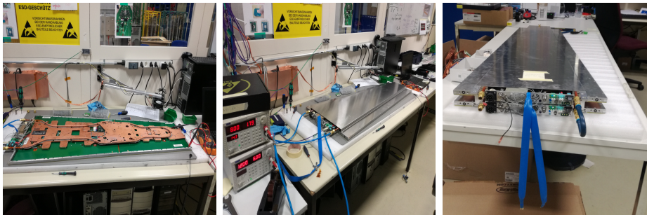
Figure 4.44: Chamber with cooling plate (left), with the thermal screen (middle), and supercavity assembly (right).
