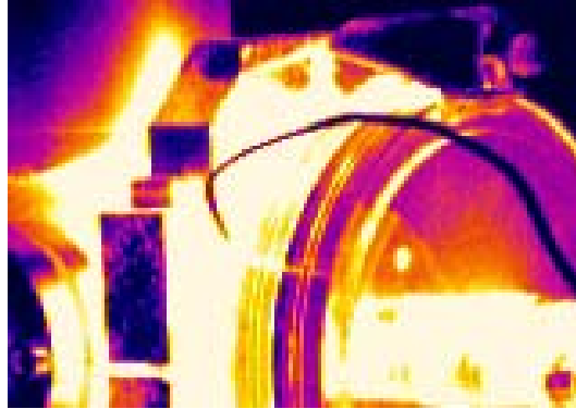
Figure 4.9: Photo taken with a thermal imager (Optris PI). One can see clearly the power feed throughs, radiating a lot of heat which leads to heating of the flange. Additionally the area where the oven is situated can be seen, as it also has quite a white glow.
