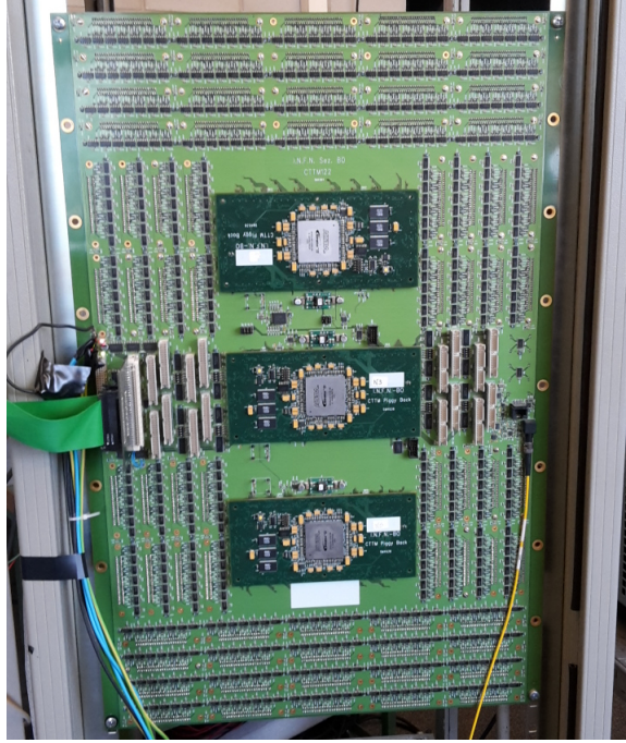
Figure 1: Front side of the CTTM board: the three FPGAs are visible. On the backside there are the LVDS connectors for the signals coming from the 72 LTM.
