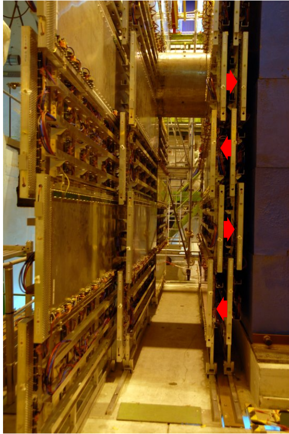
Figure 3.15: Detail of the trigger chambers installation: RPCs are placed in an alternated sequence on both sides of the supports. The red arrows show how the RPCs facing the center of the stations are moved (of about 1 cm) to better fit the electronics. For simplicity, the arrows are plotted only for MT1 but analogous considerations apply to the station MT2, shown in the “open” configuration on the left.
