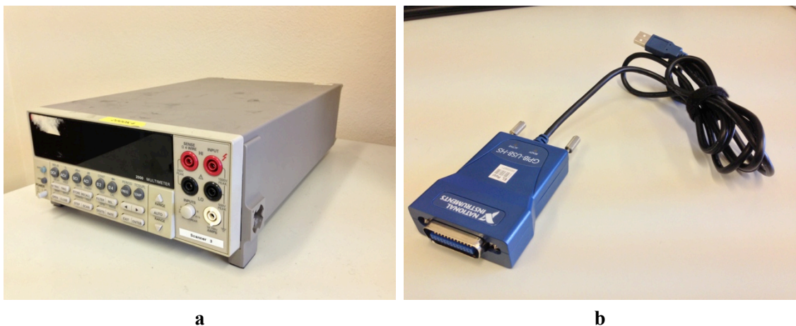
Figure 6-1 a) Keithley 2000 multimeter; b) GPIB-USB connector;
