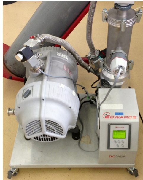
Figure 6-12 EDWARDS Vacuum pump. On the left hand side can be seen the backing pump and on the right hand side the turbomolecular pump
