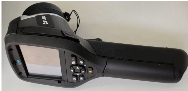
Figure 6-14 FLIR IR camera used for taking pictures of the transfer line.
