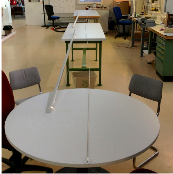
Figure 5-2 Inner pipe of the transfer line.
