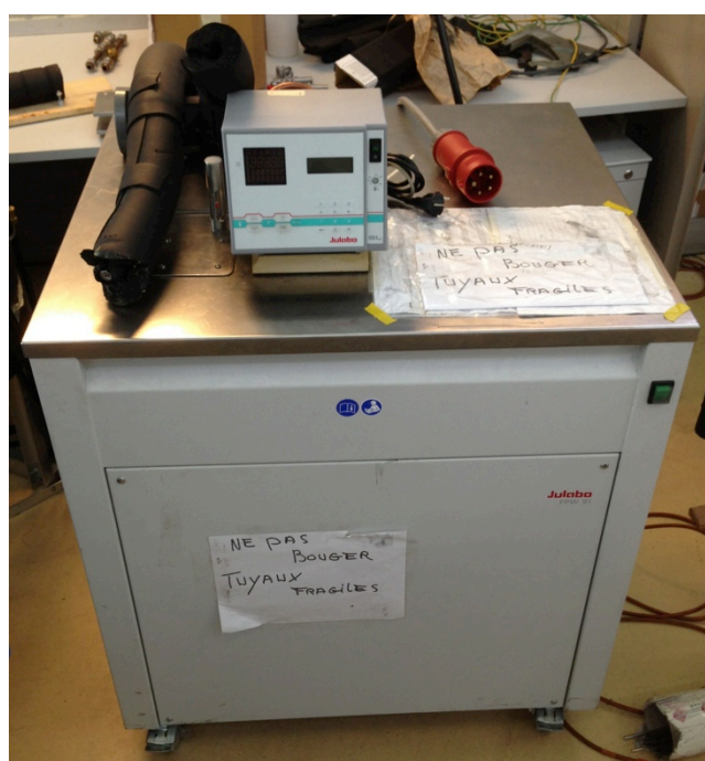
Figure 6-11 Julabo FPW 31 chiller.
