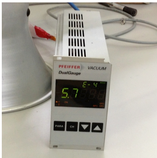
Figure 6-8 a) PFEIFFER Dual Gauge™ TPG 262 channel measurement and control unit for compact gauges; b) PFEIFFER Compact FullRange™ gauge;
