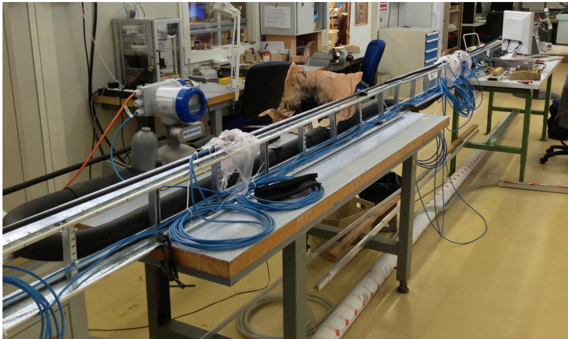
Figure 6-17 Transfer line in straight configuration with temperature sensors installed on it.
