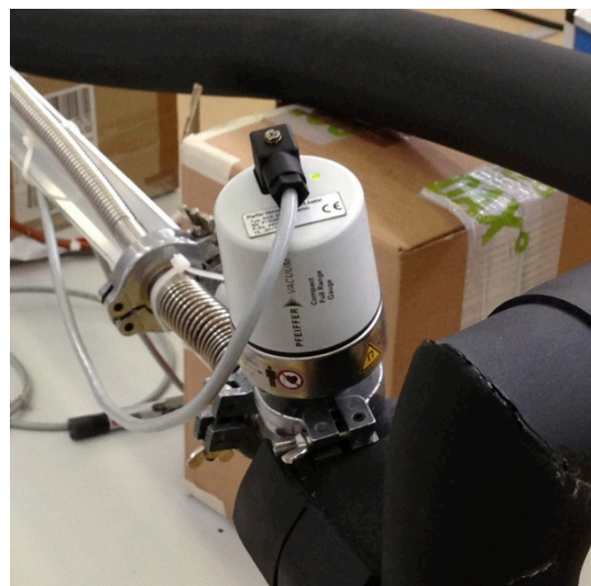
Figure 6-8 a) PFEIFFER Dual Gauge™ TPG 262 channel measurement and control unit for compact gauges; b) PFEIFFER Compact FullRange™ gauge;
