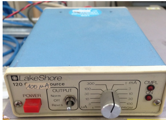
Figure 6-3 Current source used for sensors' excitation.
