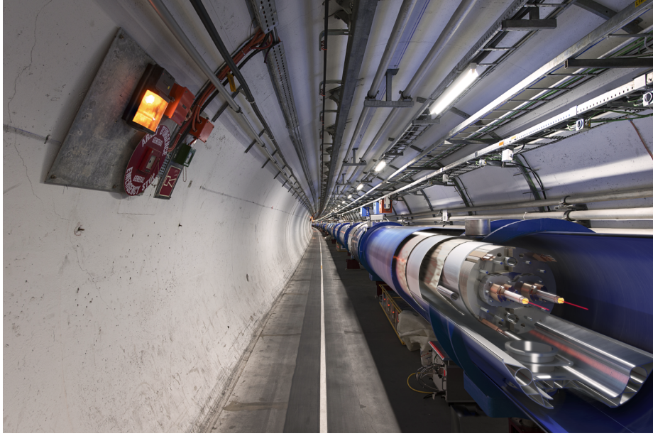
Figure 2.3: A picture of the LHC (Mobs, 2019) showing a cut of the dipole and the two beam pipes in which two sets of protons are accelerated in opposite directions (Dominguez, 2014).
