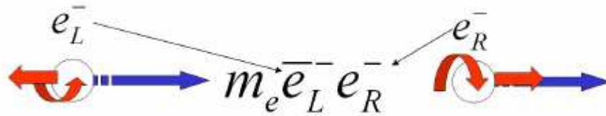
Figure 1.1: The electron Dirac mass m_e can be thought of as an interaction between a left-handed electron e_L and a right-handed electron e_R . The long (blue) arrows denote the electron momentum vector and the short (red) arrows denote the electron spin vector. For right-handed electrons e_R the spin vector and the momentum vector are aligned, whereas for left-handed electrons e_L they are opposite. The mass term may be regarded as interactions that enable left-handed electrons to interact with right-handed electrons.
