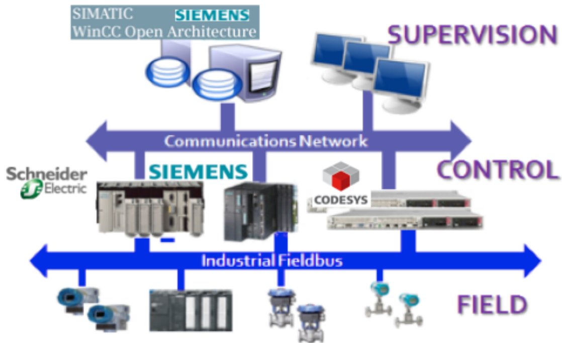
FIGURE 2.7 – CERN's UNICOS architecture [22].
