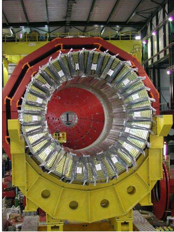
Figure 3.6: An HCAL half barrel in the assembly hall. [PTDR1]
