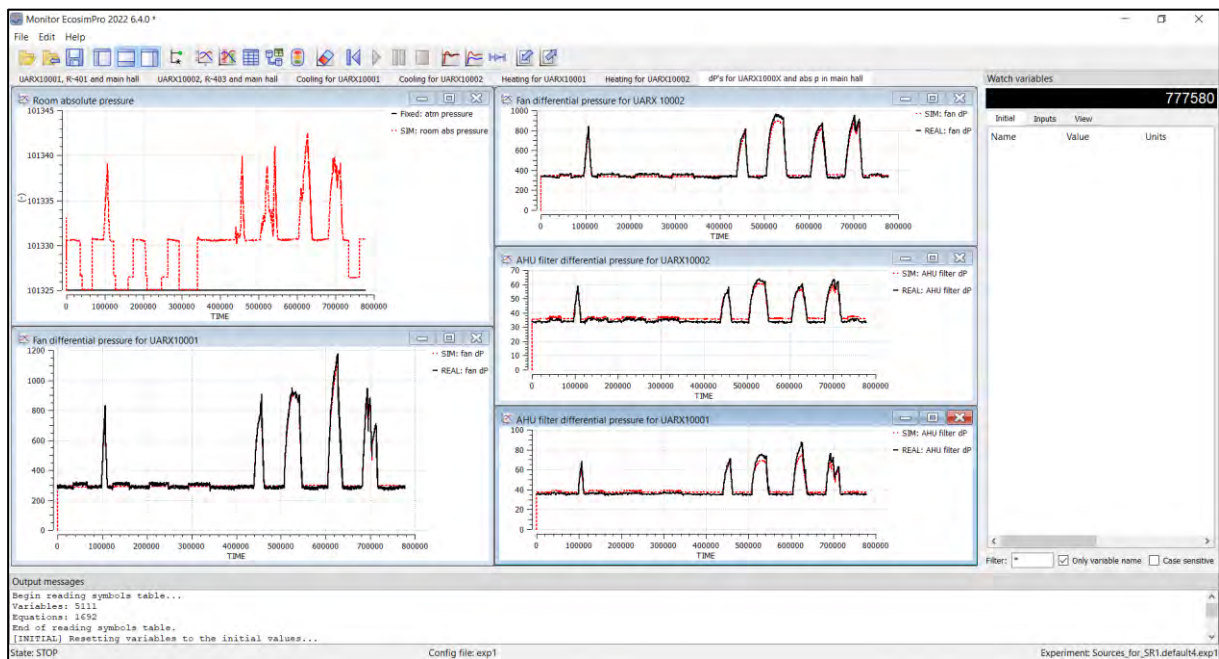
Figure 22: Screenshot of the tab: dP 's for UARX1000X and abs p in the main hall. An explanation of the containment of plots is found in the text following the figure (Own archive, 2022).
