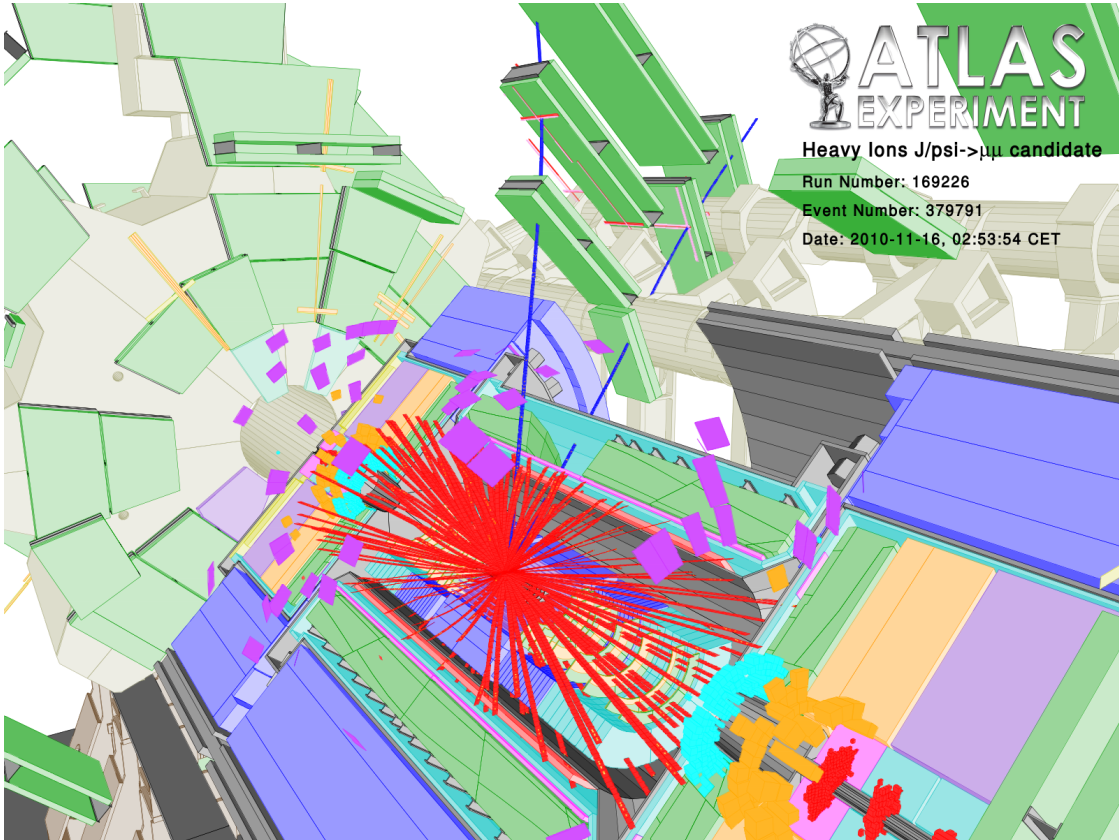
Figure 1.1: Event display of a heavy ion collision with a candidate of the decay J/\psi \rightarrow \mu^+ \mu^- . The event passes the selection requirements for J/\psi candidates in [36]. Figure taken from the event displays on [20].
