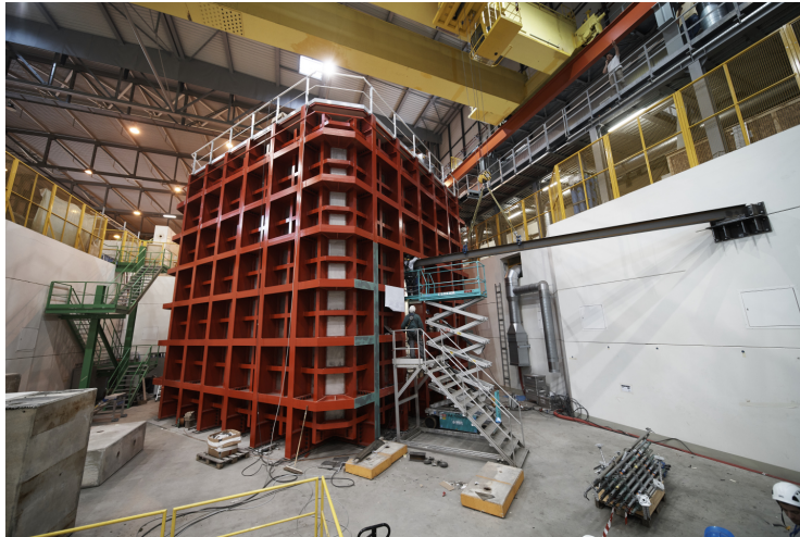
Figure 1: One of the 10x10x10m detector cubes used in protoDUNE
