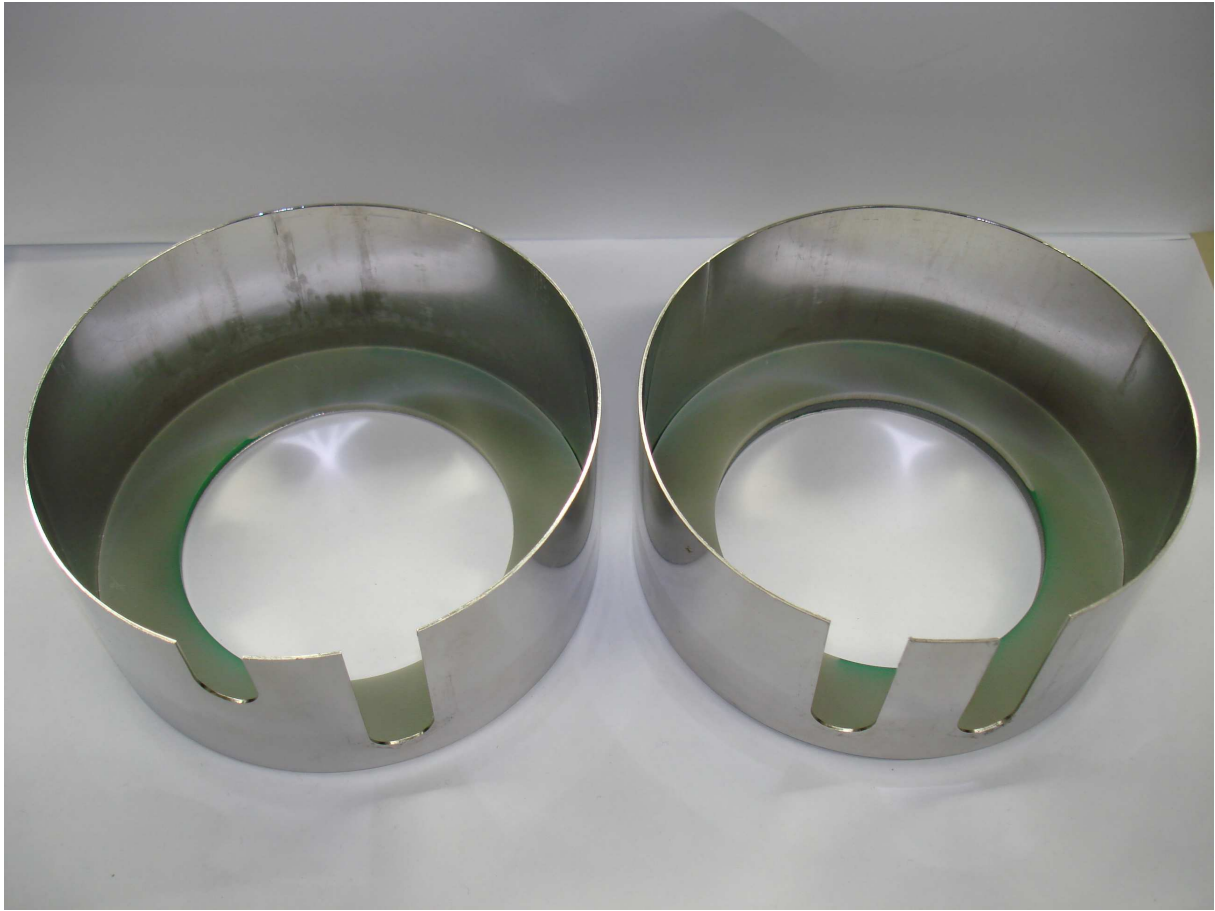
Figure 13.10: The Mu-metal static magnetic protection
