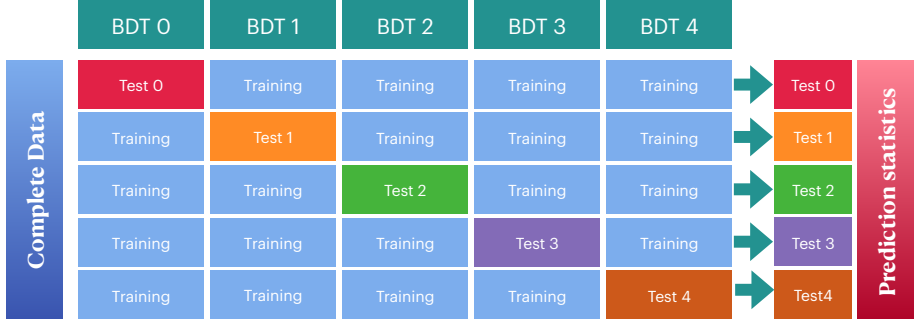
FIGURE 6.7: Representative scheme of the BDT strategy used involving 80% training and 20% testing. The events are randomly split based on their event number. This procedure is applied to obtain BDTs 0 to 4.
