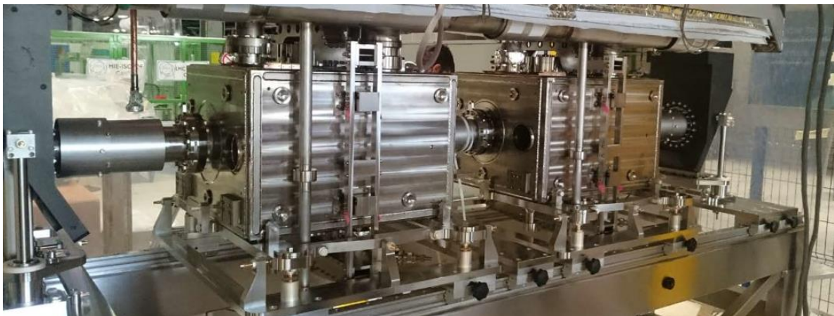
Figure 18: Two Helium vessels for DQW Crab Cavities during assembly in 2017 ©CERN
