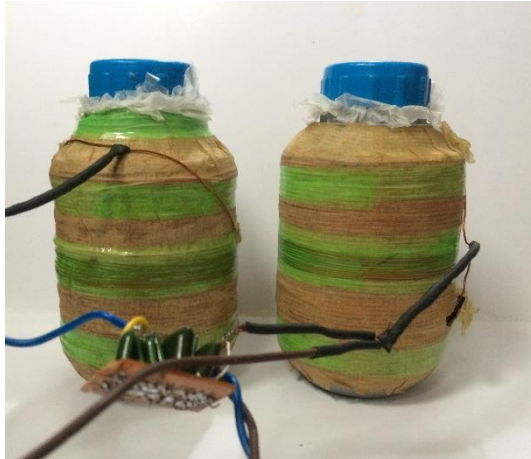
Figure IV-7 The solenoidal coils used as the magnetic sensor. They are found to be easy to wind and with high internal magnetic field uniformity. Dual solenoid configuration is used to reduce the noise.
