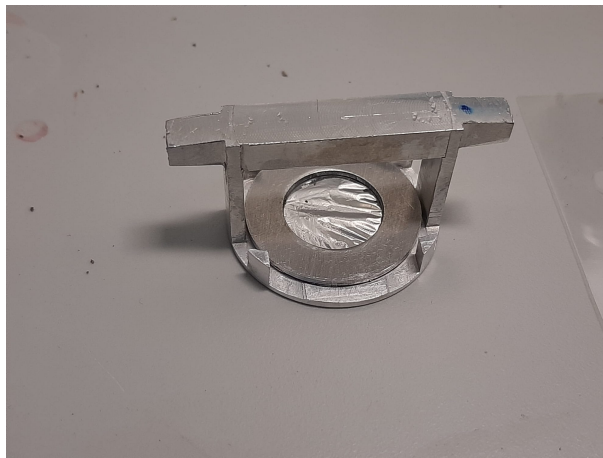
Figure 4.25: '1000' Bq source in DIRAC source holder.
