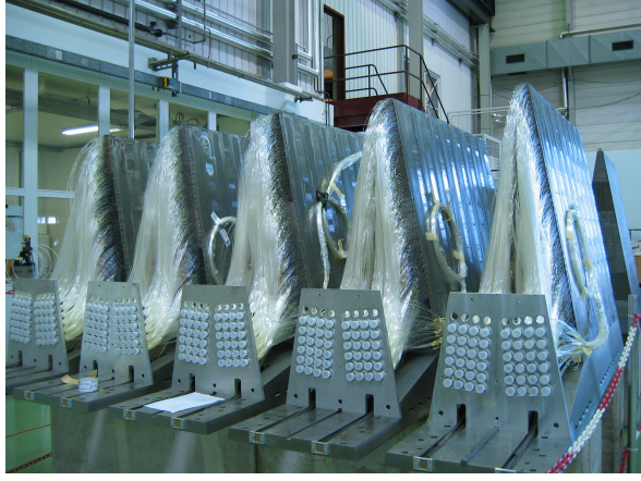
Figure 5.2. HF wedges with quartz fibres.
