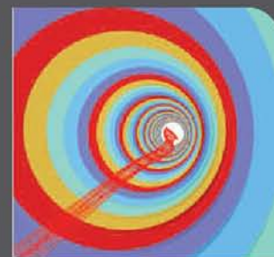
Electron trajectories through a TEM focussing stack
