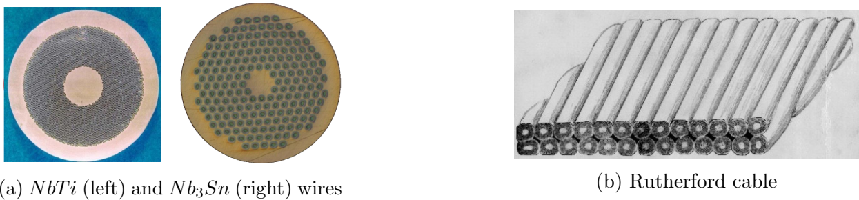
Figure 2.3: Strands and cables used for superconducting magnets (11).
