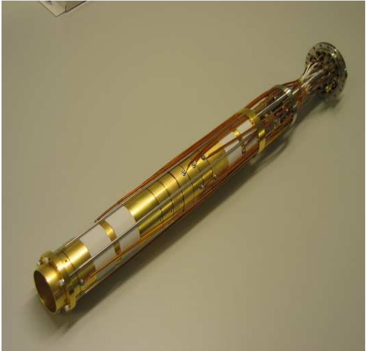
Figure 3.5: Photograph of the antiproton catching trap. The segmented electrodes can be seen with their signal wires. The two high-voltage electrodes are shown bordered by white electrical insulation.
