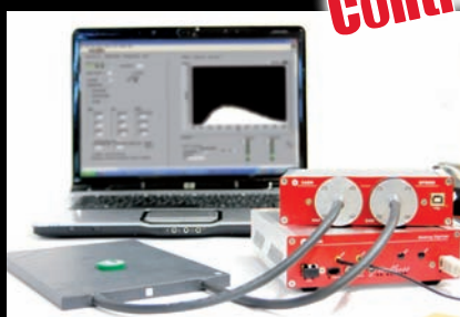
Set-up for detecting cosmic rays and \beta particles
