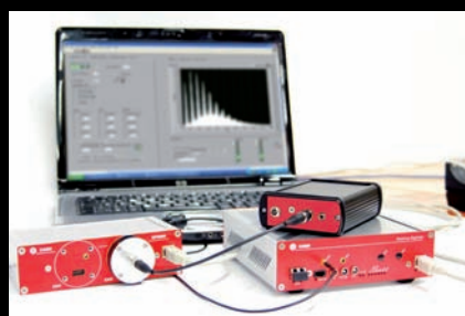
Set-up for SiPM testing & characterization
