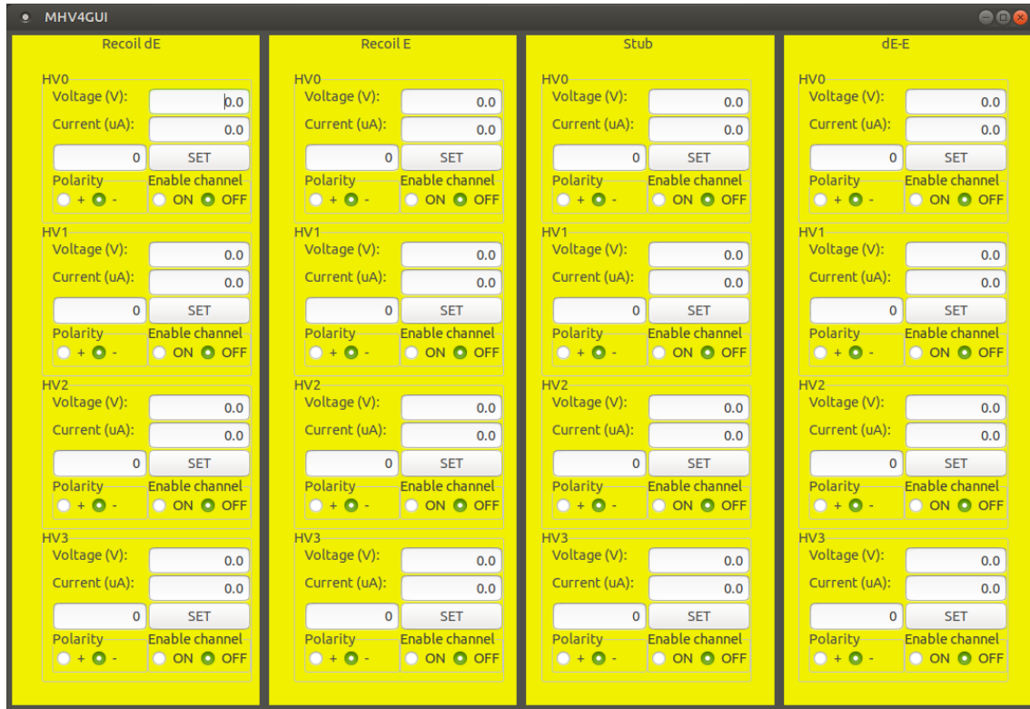
Figure 11: A screenshot of the GUI for controlling the MHV-4 units
