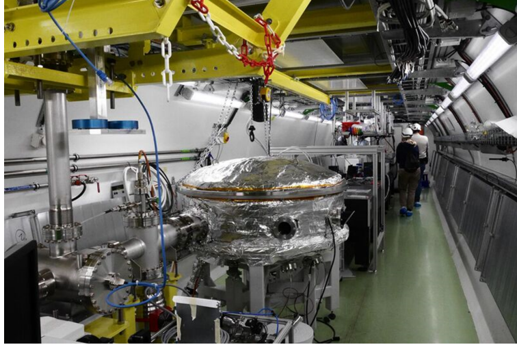
Figure 13: Photo from inside the laser room. The vacuum compressor is in the foreground, all other laser components are on the tables further back in the room. From: Ans Pardons, CERN.
