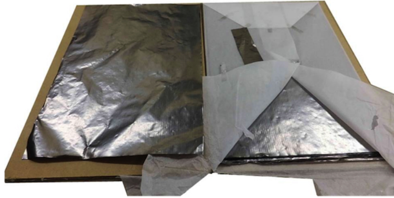
Figure 2.8: Thermal Pyrolytic Graphite (TPG) foil view. From [45].
