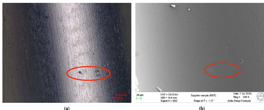
Figure B.5: Comparison of OM and SEM images at the same location in one sample. Surface features observed with the two technologies are highlighted in red. Images adapted from [185].
