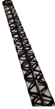
Figure 2.6: A view of a primitive ALICE ITS Upgrade module made of M55J CFRP. From [4].
