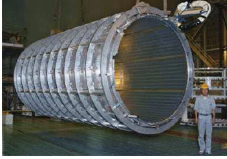
Figure 3.4: The ATLAS solenoid after completion of the coil winding [3].
