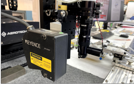
(a) A laser source LK-G157 is used to measure heights of modules for the out-of-plane metrology.
