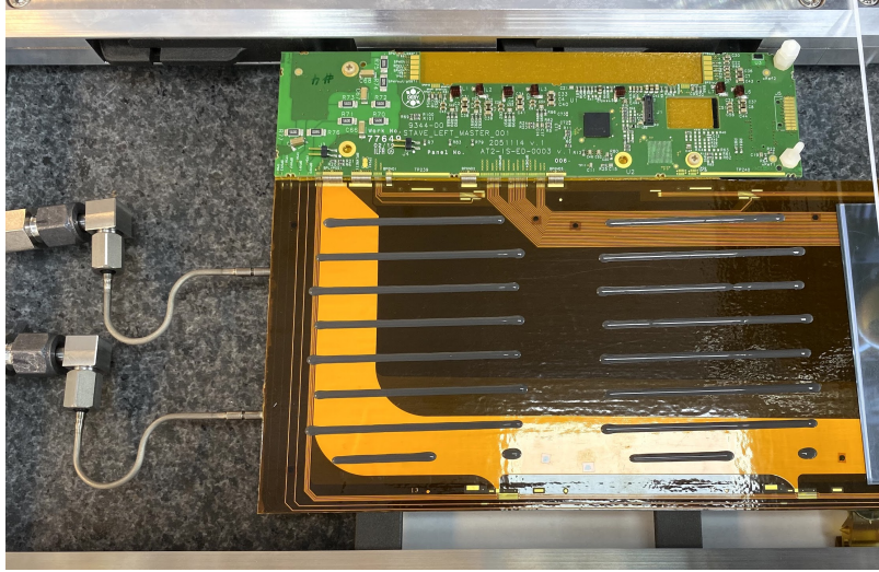
Figure 6: High z corner of a stave core with the End of Substructure master card glued down. Wirebonds connect the copper channels on the bus tape to the electrical components on the EOS. Titanium loops running through the stave core open and close on the same edge. Also shown is glue put down on the core right before electric modules are placed down.
