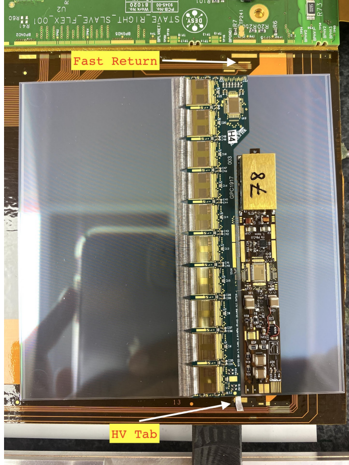
Figure 17: A number of bond pads repeat themselves 14 times over the length of the stave with the a gap of 98mm between them. Two bond pads which are used for the survey in this section are highlighted - the high voltage supply pad and the fast return ground pad.
