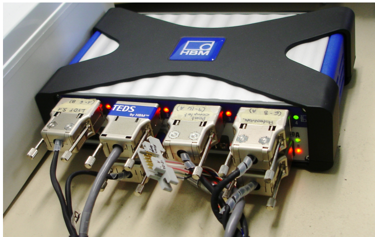
Figure 4.19.: The HBM QuantumX MX840A amplifier with 8 universal input channels.
