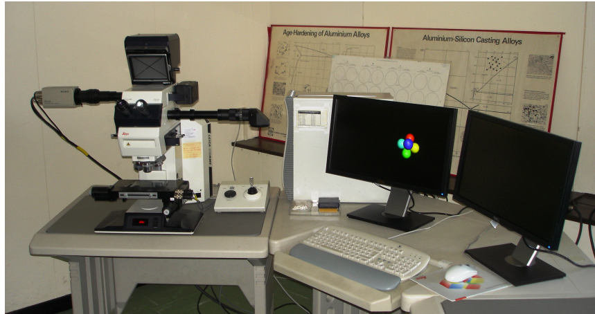
Figure 4.4.: LEICA DM RME (Quantimet-Q600) reflected light microscope, equipped with multi-lens system allowing fast swap in magnification range from 16x to 1500x (CERN).
