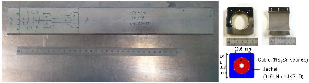
Figure 4.3.: Piece of JK2LB extruded, compacted and longitudinally strained (2.5%), circle-in-square conduit for superconductive cable with typical samples cut for metallography.
