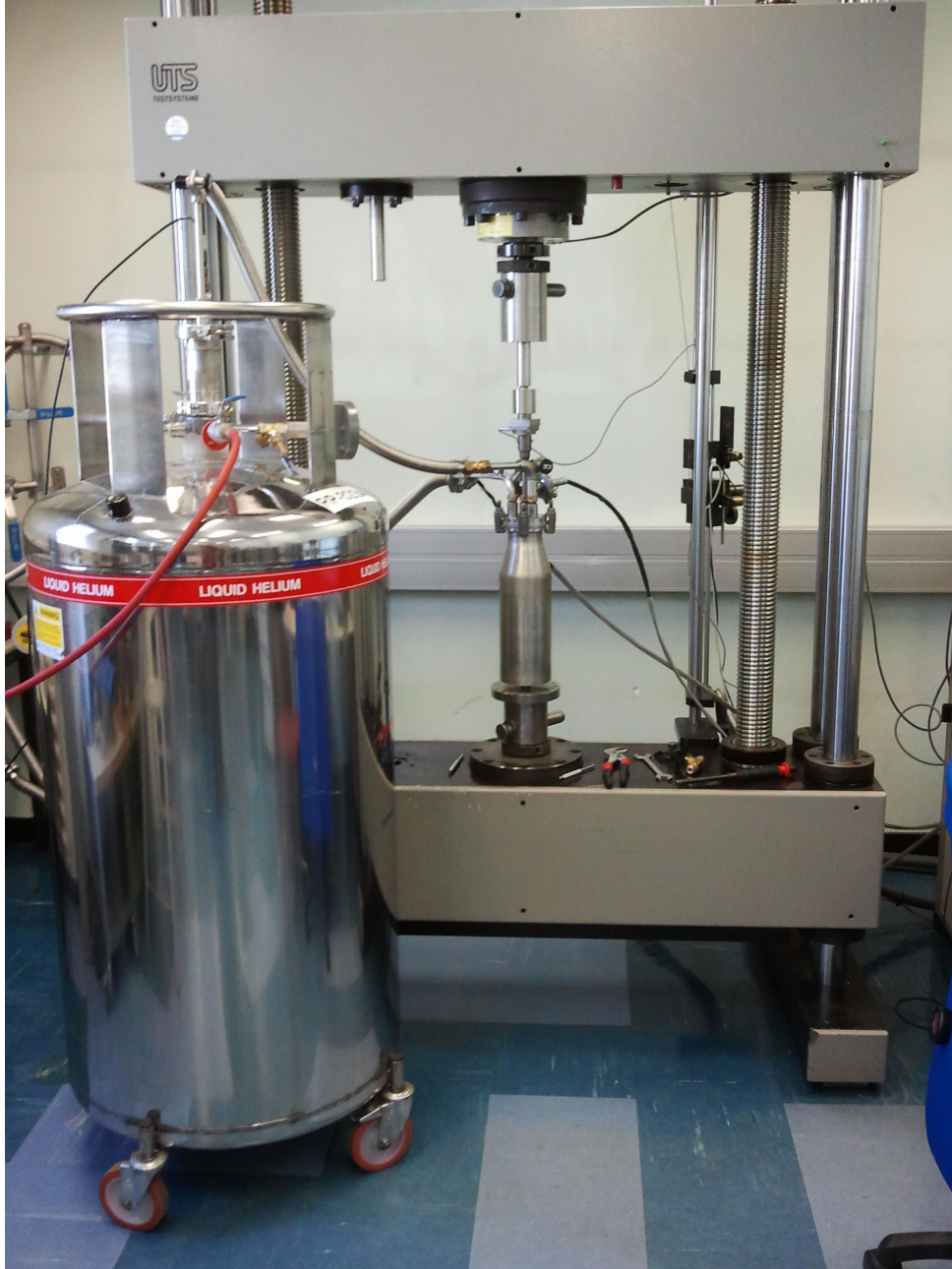
Figure 4.8.: Experimental setup placed on the UTS tensile machine.
