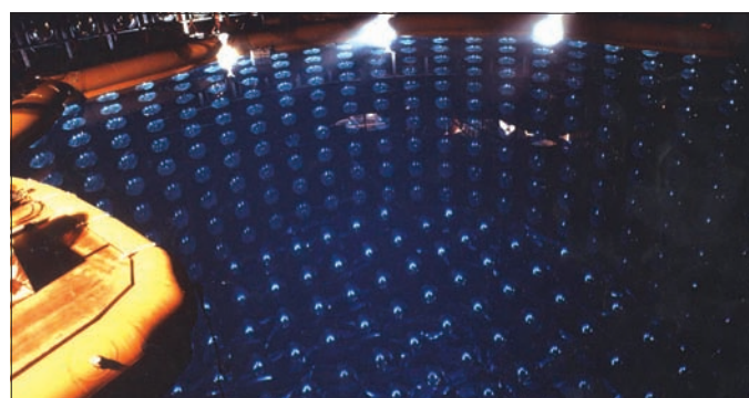
Fig. 2. A view from the top of the Kamiokande water Cherenkov detector in Japan. (Courtesy Kamiokande collaboration.)
