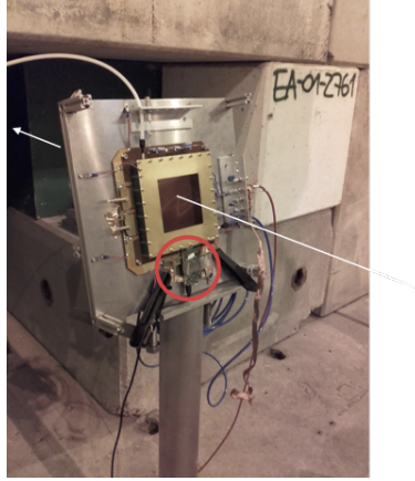
Figure 4: Set-up for the test beam in July in the North Area. One VMM3 hybrid (red circle) is connected to a standard triple GEM exposed to a muon beam (white arrow).
