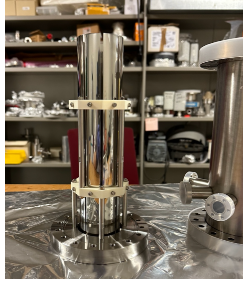
Figure 4: Photograph of the electrode structure of the octupole deflector.
